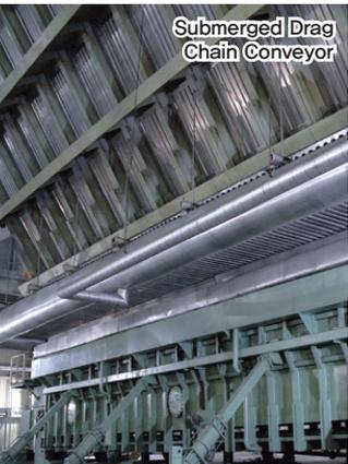
Submerged Drag Chain Conveyor
